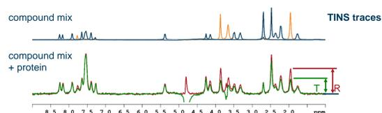
In a next step, we apply NMR in using semi-quantitative chemical shift perturbation (CSP) data to determine the binding site of the ligand in solution; and later to filter the calculated structures. The CSP study also serves to find the optimal ligand-to-protein ratio and to check for a 1:1 binding model.
